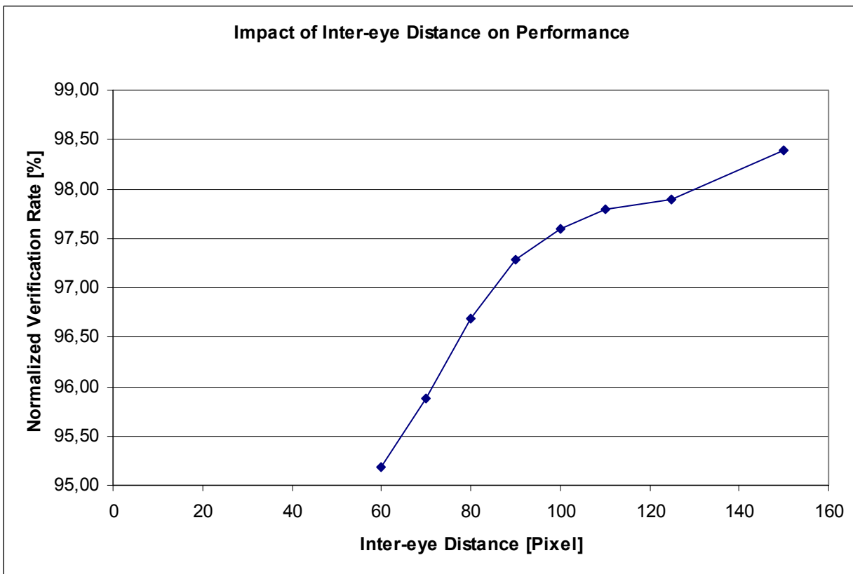
Figure 27 — Normalized verification rate plotted against inter-eye distance at FAR = 0,1 %
