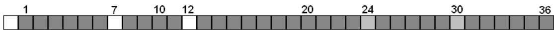
Figure M.6 — Example showing the 37 modules graded for an L side of a 36×36 module symbol
